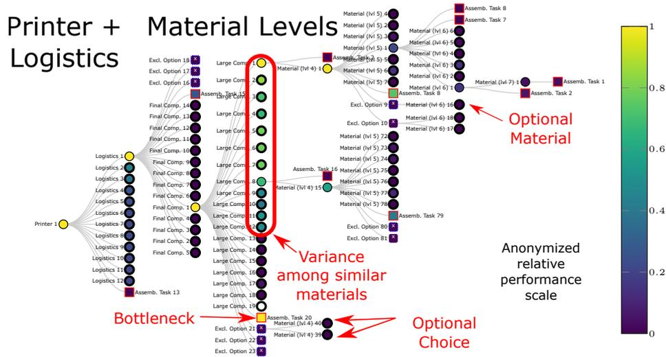
Fig. 3: Overall offset printer manufacturing process model with collapsible vertices. Each vertex corresponds to a material. Special vertices are dedicated to optional materials (blue dashed), choices (x), and assembly tasks (red vertices). The color depicts the cumulative material assembly time.
