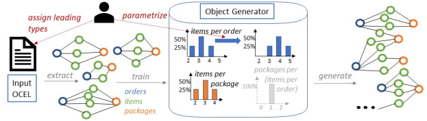
Fig. 4: By means of the leading type assignment, an OCEL (left) exhibits patterns of object relations (middle left). Based on the original or parametrized ORMDs, an object generator (middle right) can generate new sets of objects (right).
