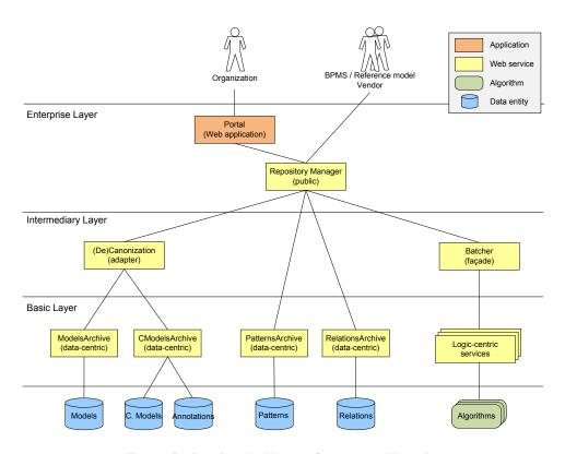
Figure 1: Service-oriented architecture of a process model repository.
