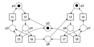
**Fig. 8.** A live and locally safe free-choice net that is not lucent because reachable markings [p3, p7, p8] and [p3, p5, p7] both enable t1 and t4.
