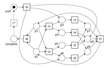
**Fig. 5.** The free-choice net without transition  $t^*$  is a workflow net. The short-circuited net is perpetual, i.e., live, bounded, and having a home cluster (e.g.,  $\{start, t0\}$ ). The short-circuited net is also lucent.
