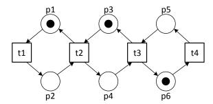
**Fig. 9.** A live and locally safe marked free-choice net that is not perpetual. The model is also not lucent since there are two reachable markings  $M_1 = [p1, p3, p6]$  and  $M_2 = [p1, p4, p6]$  that both enable t1 and t4.
