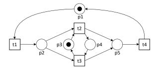
**Fig. 7.** A live and locally safe non-free-choice net. Cluster  $\{p1,t1\}$  has two reachable blocking markings  $M_1 = [p1,p3]$  and  $M_2 = [p1,p4]$ . Also cluster  $\{p5,t4\}$  has two reachable blocking markings  $M_3 = [p3,p5]$  and  $M_4 = [p4,p5]$ .
